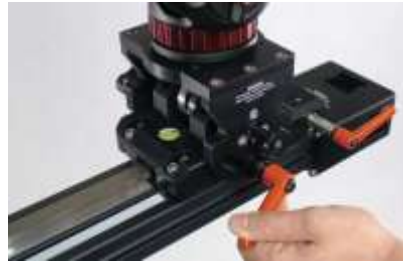
FIG 52. To disassemble the mini jib, tighten the red 'kip' handle underneath the black adjustment knob.
