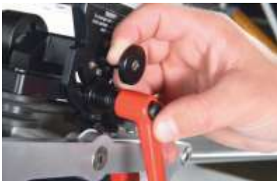
FIG 31. While holding the camera, pull out the black circular adjustment knob and position the camera in a level or desired position.
