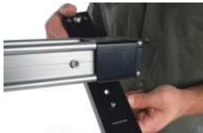
FIG 37. Attach the feet to each end of the rail using the screws provided.
