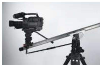
FIG 54. As the mini jib moves up and down, the camera should stay parallel with the ground.
