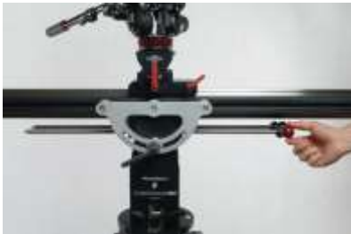
FIG 13. Remove the black nuts and the red protective balls from the counterbalance sled.
