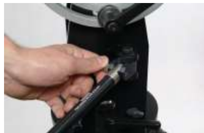
FIG 54. Once the parallelogram arm has been removed from the camera platform side, remove the opposite end on the fulcrum head.
