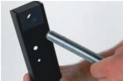
FIG 36. Insert the threaded platforms into the feet.
