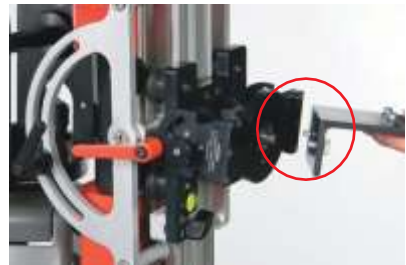
FIG 69. To mount the right angle plate, line the holes on the short side of the plate with the hole pattern on the slider platform.
