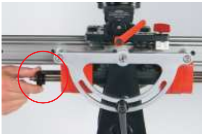
FIG 13. Reattach the black nuts for weight security.
