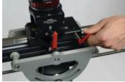
FIG 10. Loosen the red slider brake.
