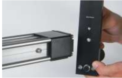
FIG 66. Add one of the feet with the threaded platforms to the side opposite the crank spline. Use the holes on the foot labeled 'Vertical Feet' and make sure the long side of the foot is facing outward.
