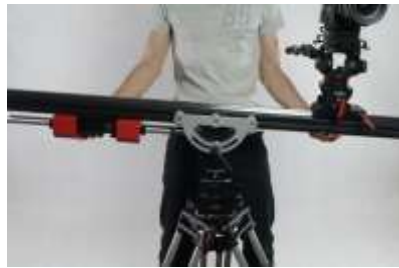
FIG 20. Hold both sides of the rail and check the balance.
