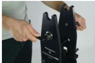
FIG 4. Remove the black 'kip' handles on each side fulcrum.
