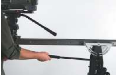
FIG 49. You may need to adjust the length of the parallelogram arm to adjust framing.
