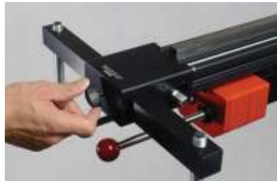
FIG 37. Lock the feet using the screws provided.
