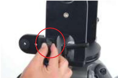
FIG 64. To mount a monitor on the fulcrum, attach one of the ears with the rubber disk facing out.
