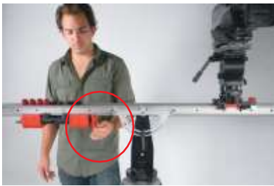
FIG 19. You may need to add or subtract counterbalance weight for precision. Repeat steps 11-18 if rebalancing is needed.
