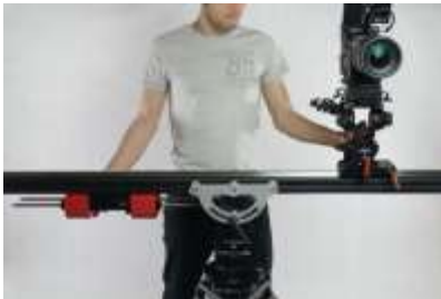
FIG 17. Slide the camera away from the center.
