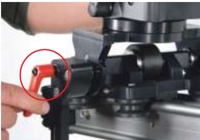
FIG 59. Remove the parallelogram lever by releasing the red 'kip' handle.
