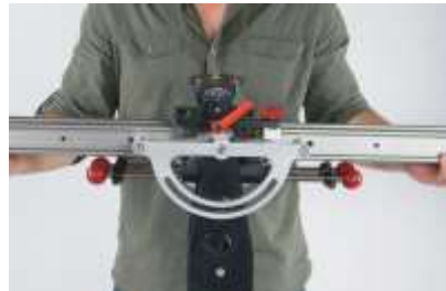
FIG 6. The 'smile' quadrant of the rail system should be on the outside of the fulcrum head.
