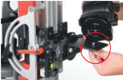
FIG 71. Mount your flat plate fluid head to the top of the right angle plate using the screw provided.
