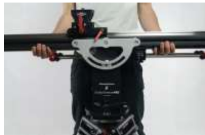
FIG 6. The 'smile' quadrant of the rail system should be on the outside of the fulcrum head.
