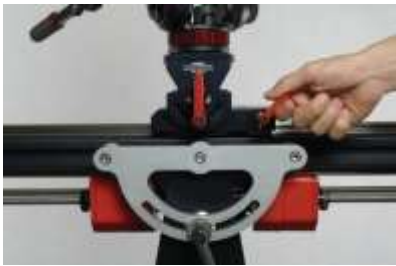
FIG 27. Apply the red slider brake handle.
