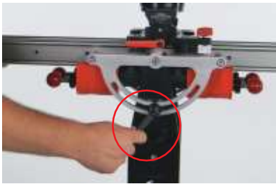
FIG 27. Loosen the black 'kip' handles on each side of the fulcrum head.
