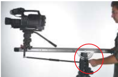
FIG 53. Release the black 'kip' handles on each side of the fulcrum head to activate the mini jib function.
