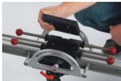
FIG 20. For camera and fluid head packages weighing more than 10kg, add the large counterweight to the bottom of the weight sled.
