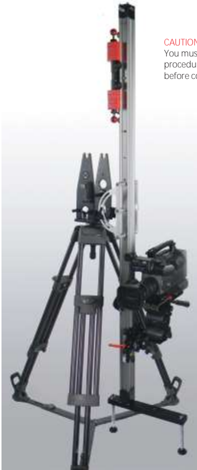
FIG 65. Complete vertical tower configuration.
