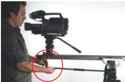
FIG 47. Attach the opposite side of the parallelogram arm to the camera platform by inserting the red 'kip' handle bolt into the threaded hole. Do not thread all the way.
