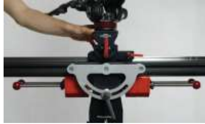
FIG 26. To angle the rail for diagonal slides, move the camera to the middle of the rail.
