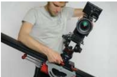
FIG 31. Hold the camera with one hand and loosen the red 'kip' handle under the black circular adjustment knob.
