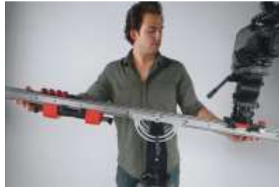
FIG 18. Hold both sides of the rail and check the balance.
