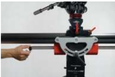
FIG 15. Reattach the black nuts for weight security.
