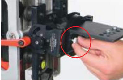
FIG 70. The long side of the plate should face up. Use the screws provided to securely mount the plate.
