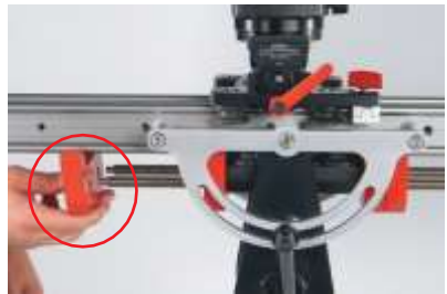
FIG 12. Add counterweight to the sled to equal the weight of the camera and fluid head package.
