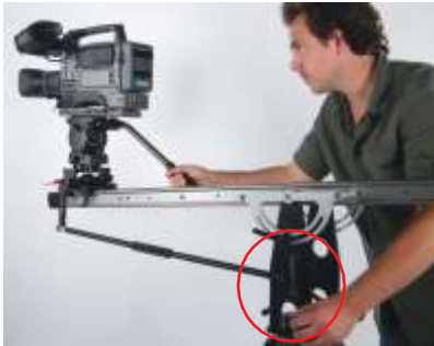
FIG 57. Loosening up the fulcrum brake handles will allow 360 degree rotations around the vertical access of the tripod.
