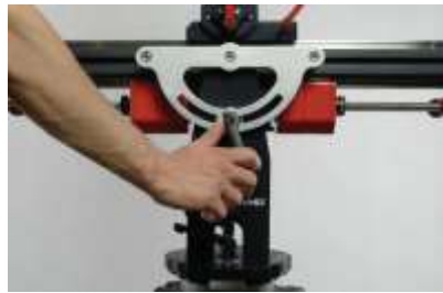
FIG 28. Loosen the black 'kip' handles on each side of the fulcrum head.
