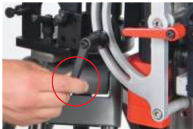
FIG 68. Add the rail in the vertical position using the black 'kip' handles from the fulcrum , threading them through the slider quadrant and into the ears previously mounted on the fulcrum.
