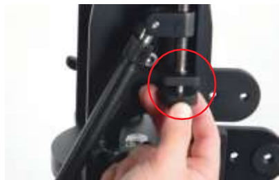
FIG 46. Turn the knob on the focal point adjustment to reposition the end of the parallelogram arm so that it is on the top of the adjustment.
