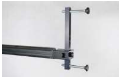
FIG 56. Add one of the feet with the threaded platforms to the side opposite the crank spline. Make sure the long side of the foot is facing outward.
