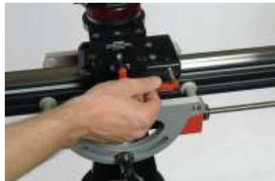
FIG 16. Loosen the red slider brake.
