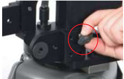
FIG 67. Add the two ears to the base of the fulcrum using the threaded knobs. Make sure the rubber disks on the ears face outward.
