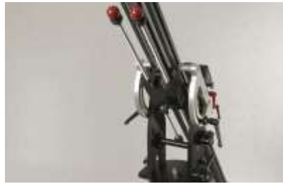
FIG 72. Remove the cup of the counterweight bearings.
