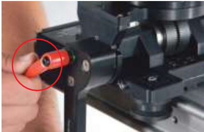
FIG 51. Complete tightening process with the red 'kip' handle. Ensure the teeth in the middle of the camera platform are fully disengaged and that the nipples on the arm's lever have fully met the holes on the platform.
