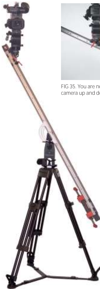
FIG 33. Once you have achieved the desired position, tighten the red 'kip' handle.
