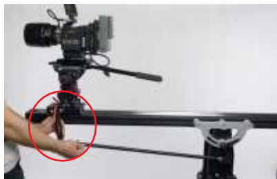
FIG 46. Attach the opposite side of the parallelogram arm to the camera platform by inserting the red 'kip' handle bolt into the threaded hole. Do not thread all the way.
