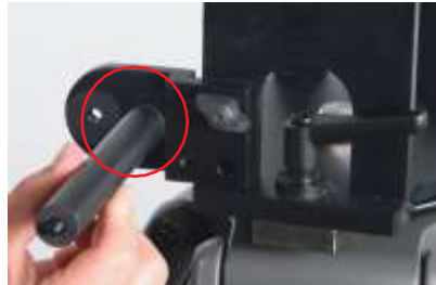
FIG 65. Attach the black mounting rod by screwing it onto the ear.
