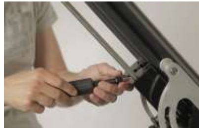
FIG 73. Grease the counterweight bearings using the grease gun provided.
