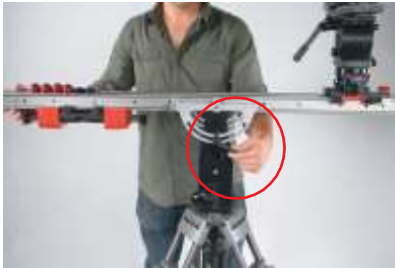
FIG 17. Loosen the black 'kip' handles on each side of the fulcrum near the rail quadrant.
