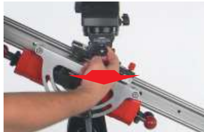
FIG 32. You will have to pull the black circular adjustment knob with great force to achieve this.
