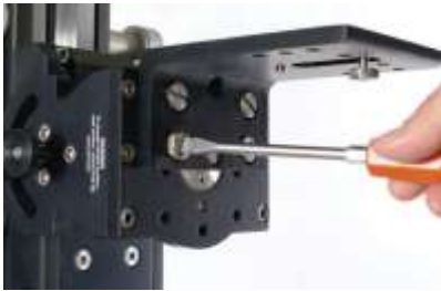
FIG 60. The long side of the plate should face up. Use the screws provided to securely mount the plate.
